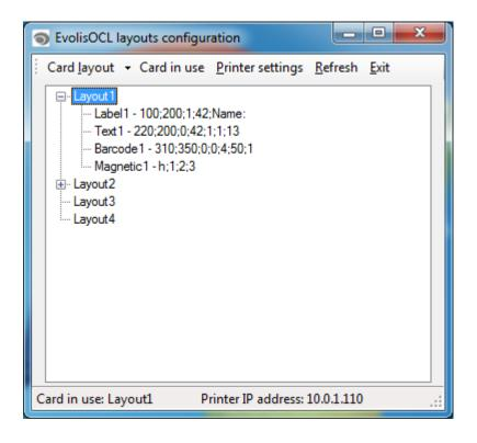
The "Card layout" menu is used to add, edit and delete the objects, like text, labels, barcodes and magnetic encoding.
